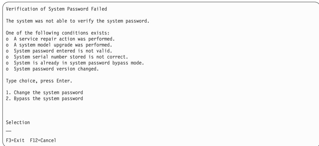
Figure 69. Example of the Verification of System Password Failed display
